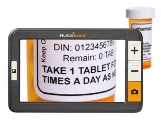
**EyePal Solo OCR** – Stand-alone scanning and reading equipment with optical character recognition and read-aloud capabilities.
